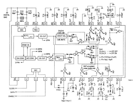
Notes: 1. The items D1 through D10 in the figure indicate points that are switched by the serial data. 2. Use capacitors with good high-frequency characteristics for the capacitors on pins 7, 14, and 22. Also, connect 0.1-µF ceramic capacitors in parallel.
