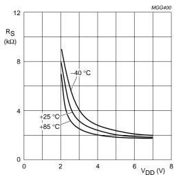
b. Segment output impedance S0 to S23 (R<sub>S</sub>);  $V_{DD} = 5 \text{ V}.$
