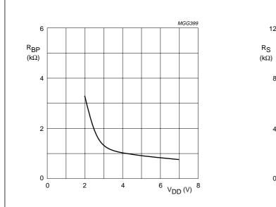
a. Backplane output impedance BP0 to BP3 (R<sub>BP</sub>);  $V_{DD}$  = 5 V;  $T_{amb}$  = -40 to +85 °C.
