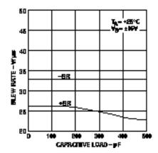
Slew Rate vs. Capacitive Load
