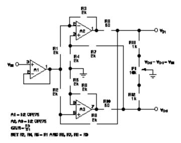
Figure 17. High Speed, Low Noise Differential Line Driver
