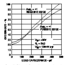
Small-Signal Overshoot vs. Load Capacitance
