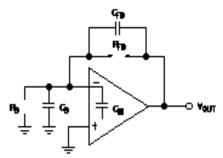
Figure 14. Compensating the Feedback Pole
