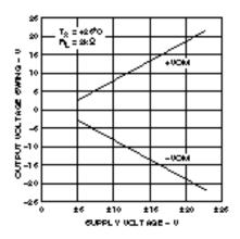
Output Voltage Swing vs. Supply Voltage
