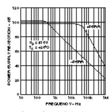
Power Supply Rejection vs. Frequency
