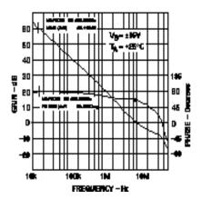
Open-Loop Gain, Phase vs. Frequency
