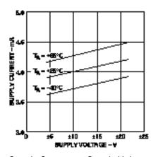
Supply Current vs. Supply Voltage
