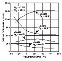
Open-Loop Gain vs. Temperature
