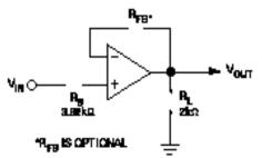
Figure 9. Output Voltage Phase Reversal Fix
