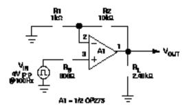
Figure 10. Overload Recovery Time Test Circuit
