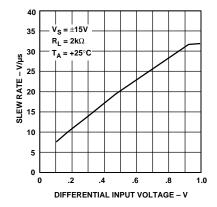
Slew Rate vs. Differential Input Voltage
