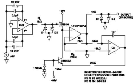
Figure 11. OP275's Settling Time Test Fixture
