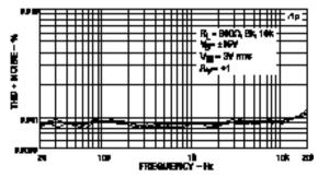
Figure 2. THD + Noise vs. Frequency vs. R<sub>LOAD</sub>
