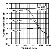
Closed-Loop Gain vs. Frequency
