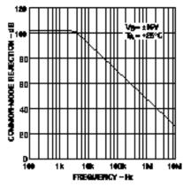
Common-Mode Rejection vs. Frequency
