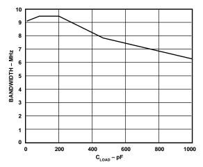
Figure 16. Bandwidth vs. CLOAD
