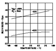
Slew Rate vs. Temperature
