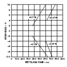
Settling Time vs. Step Size
