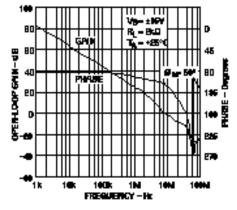
Open-Loop Gain, Phase vs. Frequency
