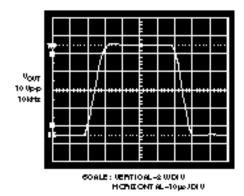
Figure 19. Low-Pass Filter Transient Response
