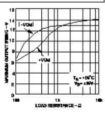
Maximum Output Voltage vs. Load Resistance
