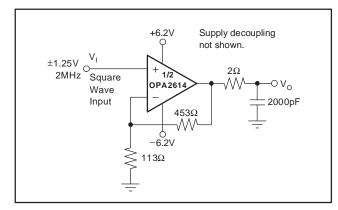
Figure 15. Large Capacitive Load Driver
