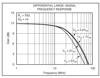
Figure 6. OPA2613 Differential Gain of +4 Large-Signal Bandwidth
