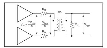
Figure 11. Driver Peak Output Voltage
