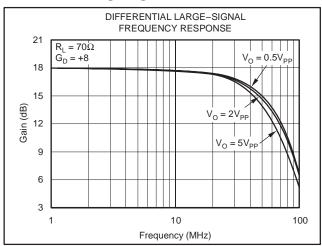
Figure 7. OPA2614 Differential Gain of +8 Large-Signal Bandwidth
