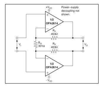
Figure 5. Noninverting Differential I/O Amplifier
