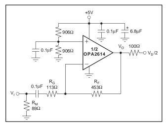
Figure 4. AC-Coupled, G = -4, Single-Supply, Specification and Test Circuit
