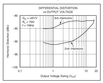
Figure 9. OPA2614 Differential Gain of +8 Distortion vs Output at 1MHz
