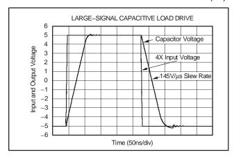
Figure 16. Large-Signal Capacitive Load Drive
