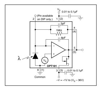
FIGURE 2. Bipolar Power Supply Circuit Connections.
