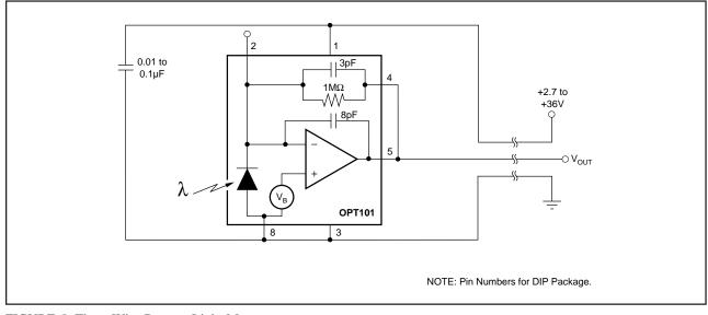
FIGURE 5. Three-Wire Remote Light Measurement.
