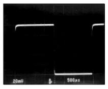
$\begin{array}{l} \mbox{SMALL SIGNAL RESPONSE (C_{LOAD} = 10,000 \mbox{ pF})} \\ (\mbox{Pin 3 = 0V}) \end{array}$
