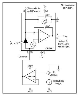
FIGURE 3. Dark Error (Offset) Adjustment Circuit.
