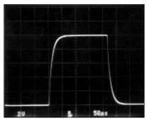
$\begin{array}{l} \mbox{SMALL SIGNAL RESPONSE (C_{LOAD} = 10,000 \mbox{ pF})} \\ (\mbox{Pin } 3 = -15 \mbox{V}) \end{array}$
