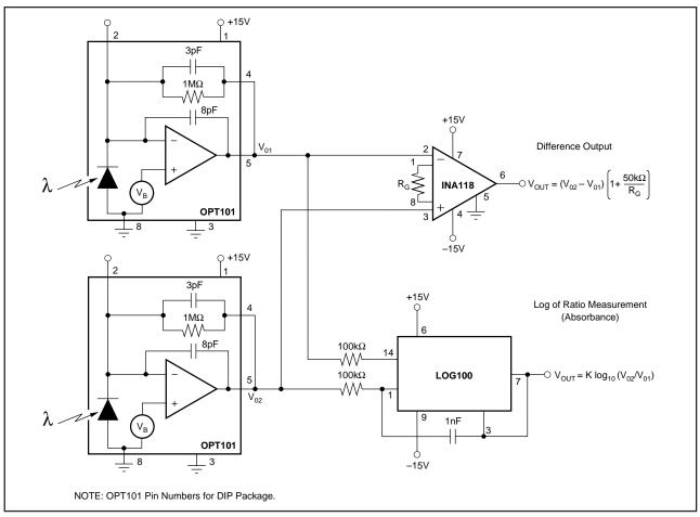
FIGURE 6. Differential Light Measurement.
