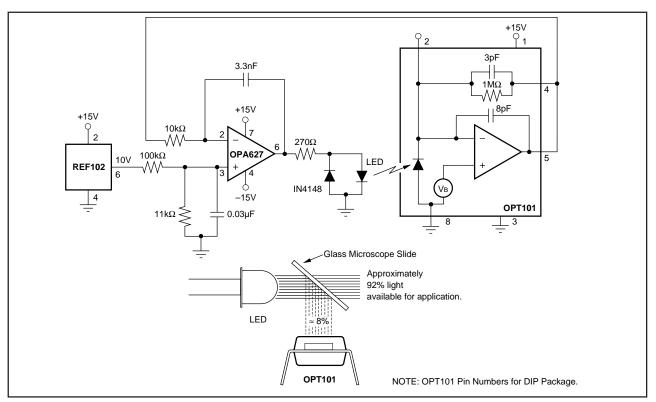
FIGURE 7. LED Output Regulation Circuit.
