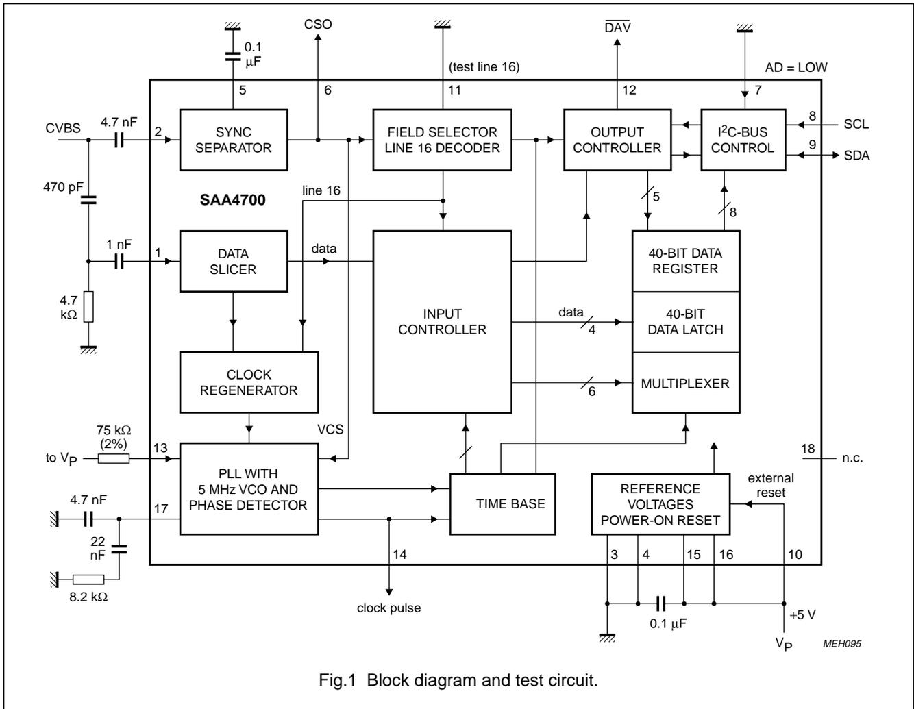
Fig.1 Block diagram and test circuit.
