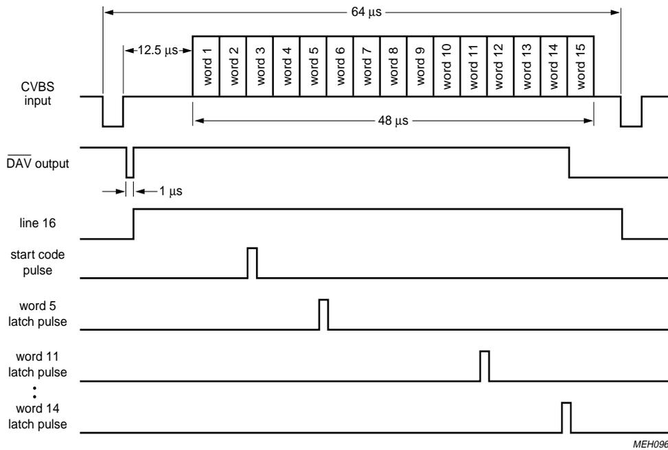
Fig.5 Timing diagram of the data available output and word latch pulses.
