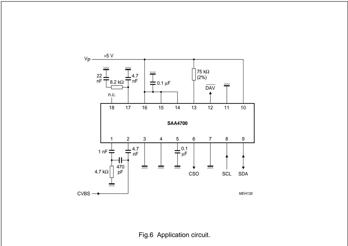
Fig.6 Application circuit.
