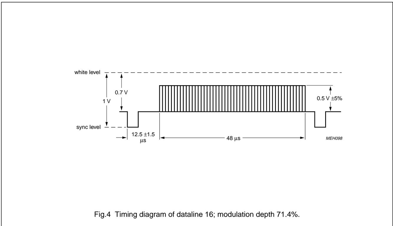
Fig.4 Timing diagram of dataline 16; modulation depth 71.4%.
