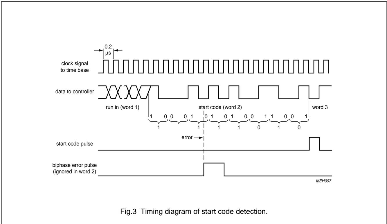
Fig.3 Timing diagram of start code detection.
