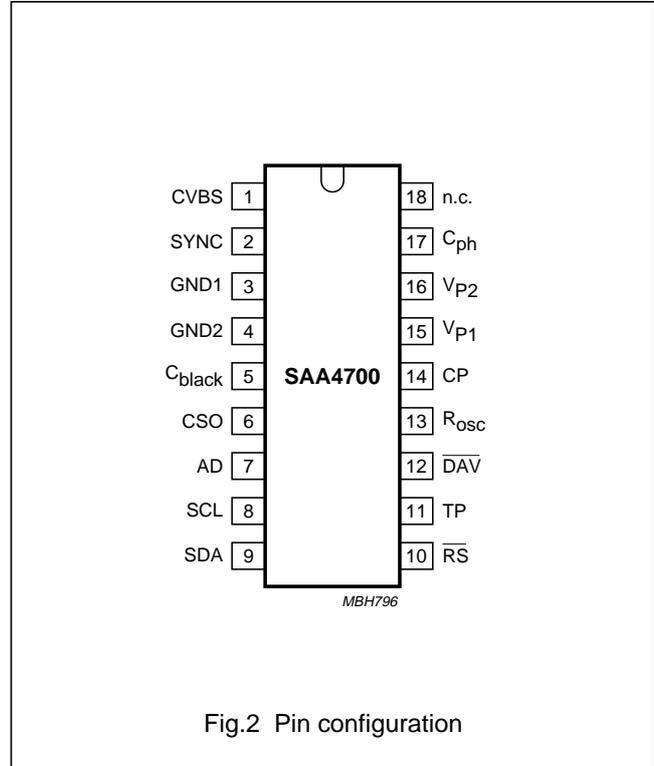
Fig.2 Pin configuration
