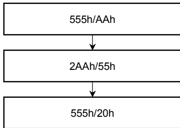
Fast Program Set Command Sequence (address/data)
