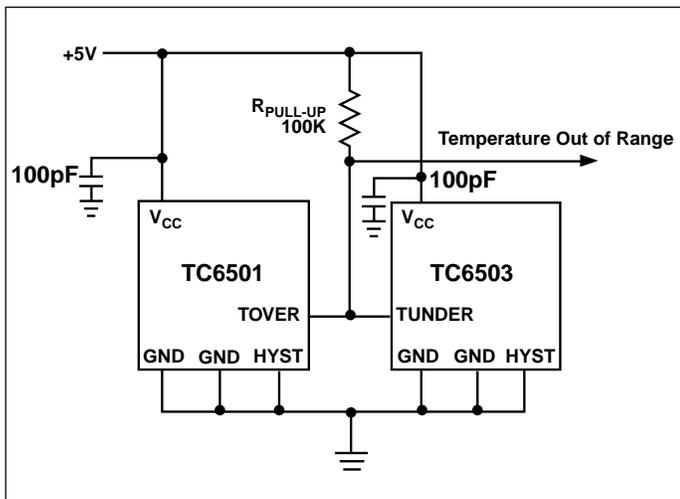
Figure 1. Over and Under Temperature Alarm
