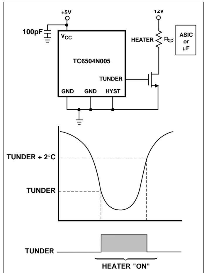
Figure 3. TC6504N005 As Heater Thermostat
