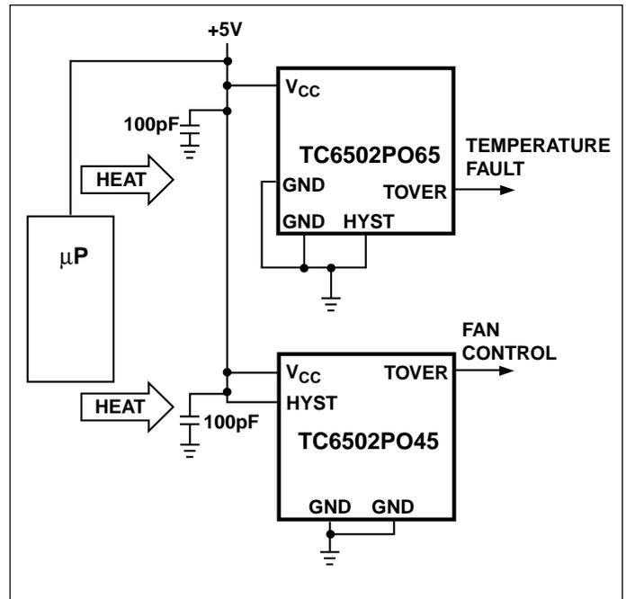
Figure 2. Fan Control Circuit with Over Temperature Alert
