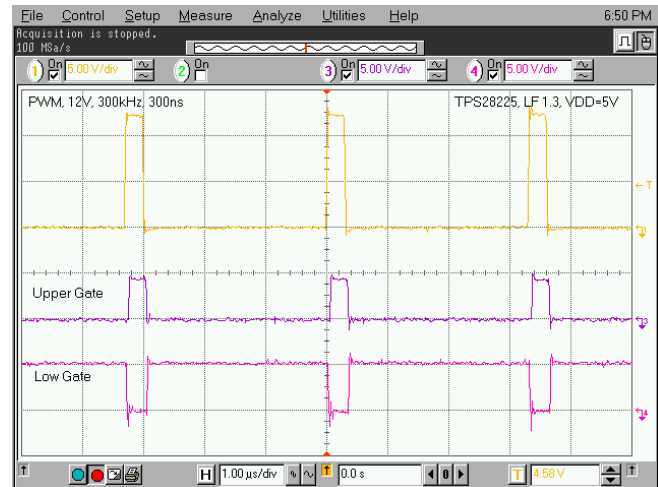
Figure 26. 12-V PWM Pulse at V_{DD} = 5 V
