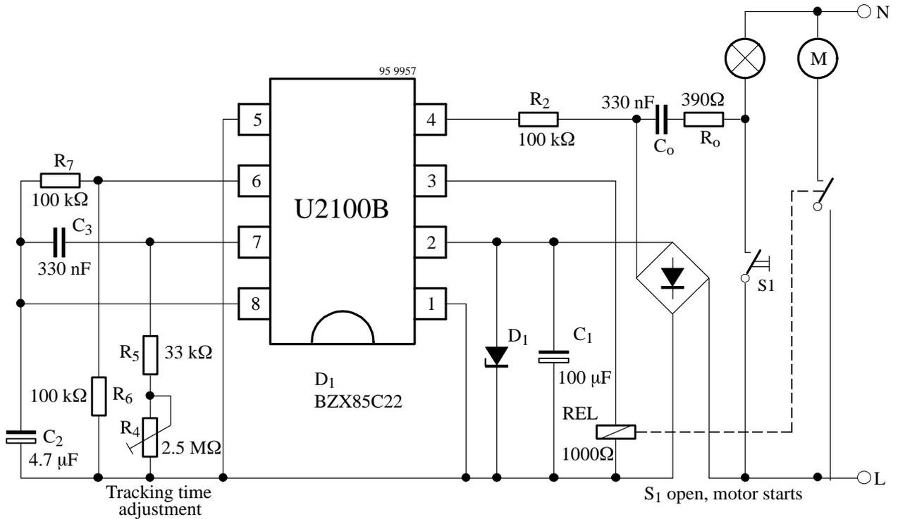
Figure 10. Fan tracking time control 18 sec. to 23 min.
