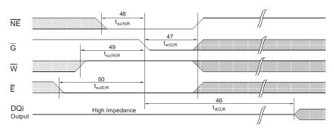
r: If  $\overline{W}$  is LOW at any point in which both  $\overline{E}$  and  $\overline{NE}$  are LOW and  $\overline{G}$  is HIGH, than a STORE cycle will be initiated instead of a RECALL.
