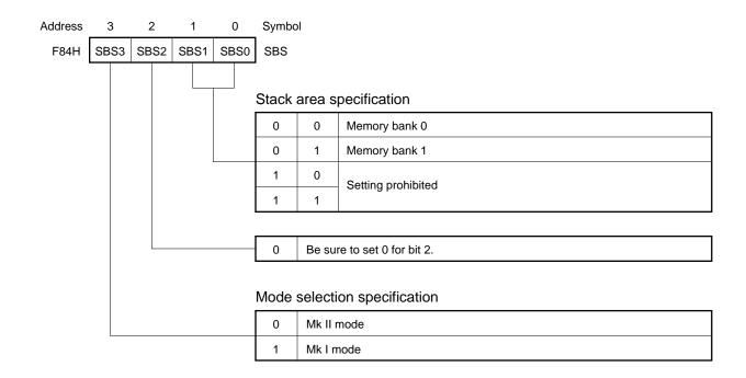
Caution SBS3 is set to "1" after RESET input, and consequently the CPU operates in the Mk I mode. When using instructions for the Mk II mode, set SBS3 to "0" to enter the Mk II mode before using the instructions.
