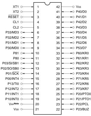
**Note** Directly connect VPP to VDD in the normal operation mode.
