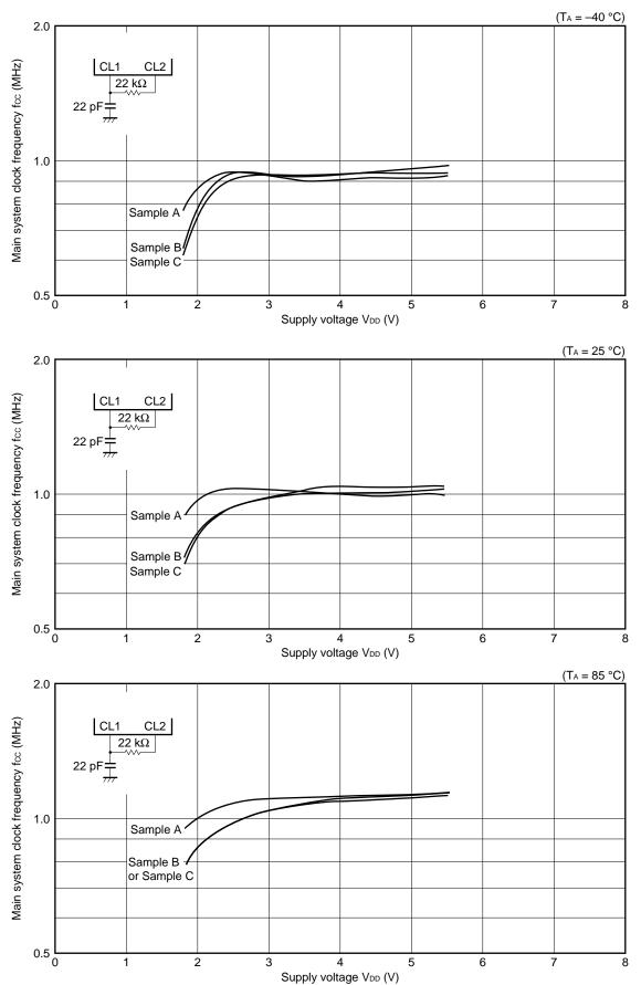
fcc vs Ta (RC oscillation, R = 22k $\Omega$ , C = 22 pF)
