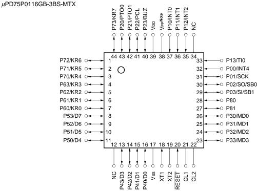
**Note** Directly connect VPP to VDD in the normal operation mode.
