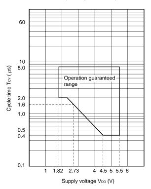
(2) Serial interface channel 0 (T<sub>A</sub> = -40 to +85°, V<sub>DD</sub> = 1.8 to 5.5 V)
