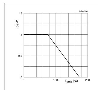
Fig.2 Maximum forward current as a function of ambient temperature.
