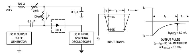
Notes: 1. A 2.0 k $\Omega$  variable resistor adjusted for a Forward Current (I<sub>F</sub>) of 30 mA.
