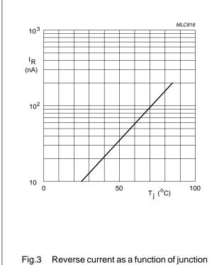
Fig.3 Reverse current as a function of junction temperature; maximum values.
