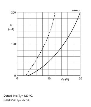
Fig.5 Forward current as a function of maximum forward voltage.
