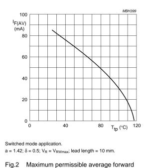
current as a function of tie-point temperature (including losses due to reverse leakage).
