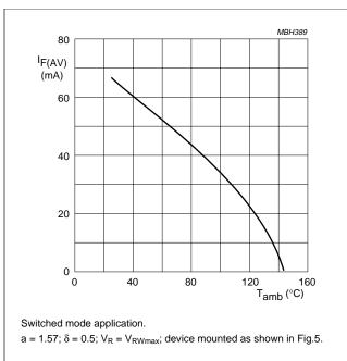
Fig.2 Maximum permissible average forward current as a function of ambient temperature (including losses due to reverse leakage).
