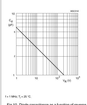
Fig.10 Diode capacitance as a function of reverse voltage; typical values.
