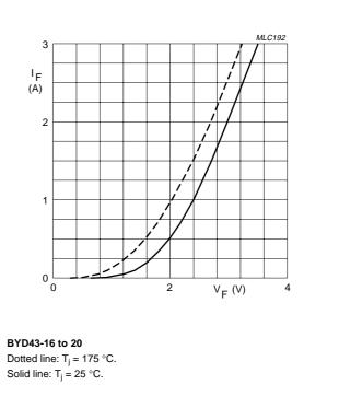
Fig.15 Forward current as a function of forward voltage; maximum values.
