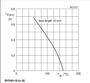
$a = 1.42; \ V_R = V_{RRMmax}; \ \delta = 0.5.$  Switched mode application.
