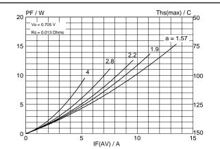
Fig.4. Maximum forward dissipation  $P_F = f(I_{F(AV)})$  per diode; sinusoidal current waveform where a = form factor  $= I_{F(RMS)} / I_{F(AV)}$ .
