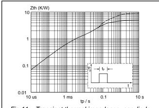
Fig.11. Transient thermal impedance; per diode;  $Z_{th j-hs} = f(t_p)$ .
