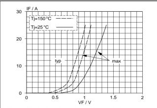
Fig.9. Typical and maximum forward characteristic  $I_F = f(V_F)$ ; parameter  $T_j$
