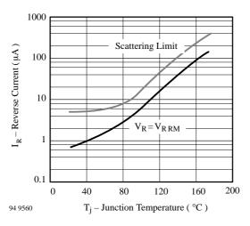
Figure 5. Reverse Current vs. Junction Temperature
