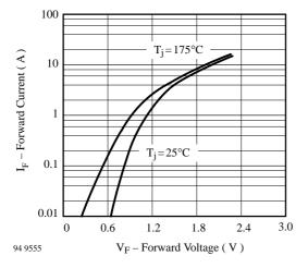
Figure 6. Forward Current vs. Forward Voltage
