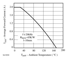
Figure 4. Average Forward Current vs. Ambient Temperature
