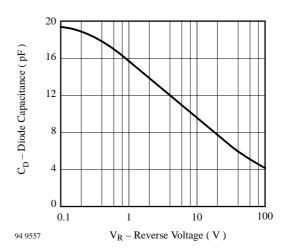
Figure 7. Diode Capacitance vs. Reverse Voltage
