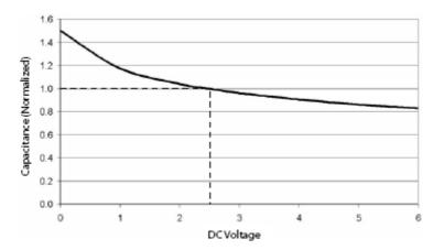
Figure 1. Diode Capacitance vs. Reverse Voltage
