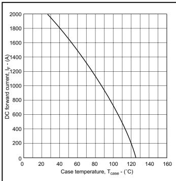
Fig. 6DC current rating vs case temperature
