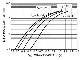
Figure 1. Typical Forward Voltage
