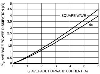
Figure 7. Forward Power Dissipation
