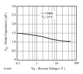
Figure 7. Diode Capacitance vs. Reverse Voltage
