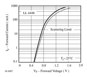
Figure 5. Forward Current vs. Forward Voltage
