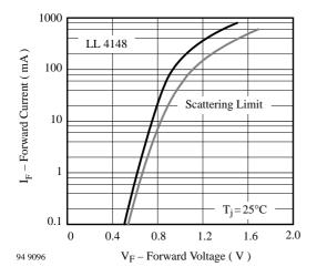
Figure 4. Forward Current vs. Forward Voltage
