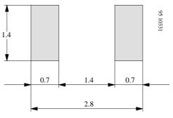
Figure 3. Recommended foot pads (in mm)
