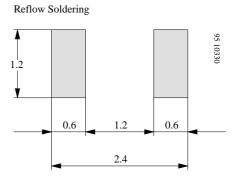
Figure 2. Recommended foot pads (in mm)
