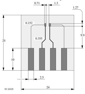
Figure 1. Board for  $R_{thJA}$  definition (in mm)
