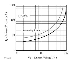
Figure 6. Reverse Current vs. Reverse Voltage
