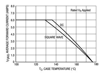
Figure 3. Total Device Current Derating, Case
