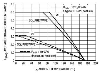
Figure 4. Total Device Current Derating, Ambient
