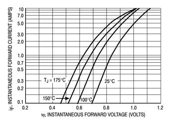
Figure 1. Typical Forward Voltage
