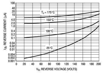
Figure 2. Typical Reverse Current
