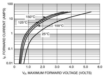
Figure 1. Typical Forward Voltage
