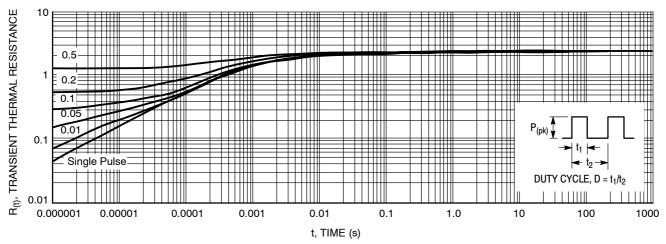
Figure 8. Thermal Response, Junction to Case
