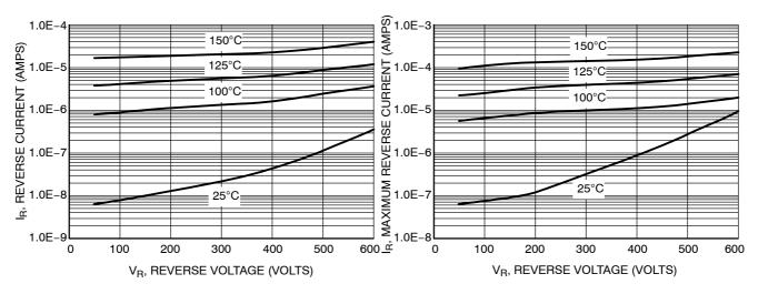
**Figure 3. Typical Reverse Current**
