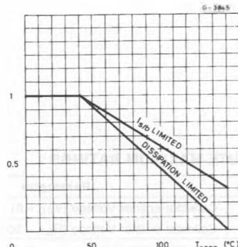
I - Area of permissible operation during Turn-on provided  $R_{BE} \leq 100\text{ }\Omega$  and  $t_p \leq 0.6\text{ }\mu\text{s}$ .
