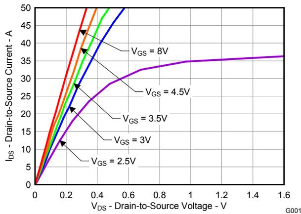
**Figure 2. Saturation Characteristics**
