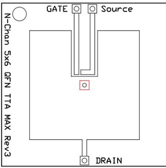
Max  $R_{\theta JA} = 51^\circ\text{C/W}$
