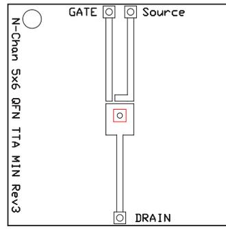
Max  $R_{\theta JA} = 125^\circ\text{C/W}$
