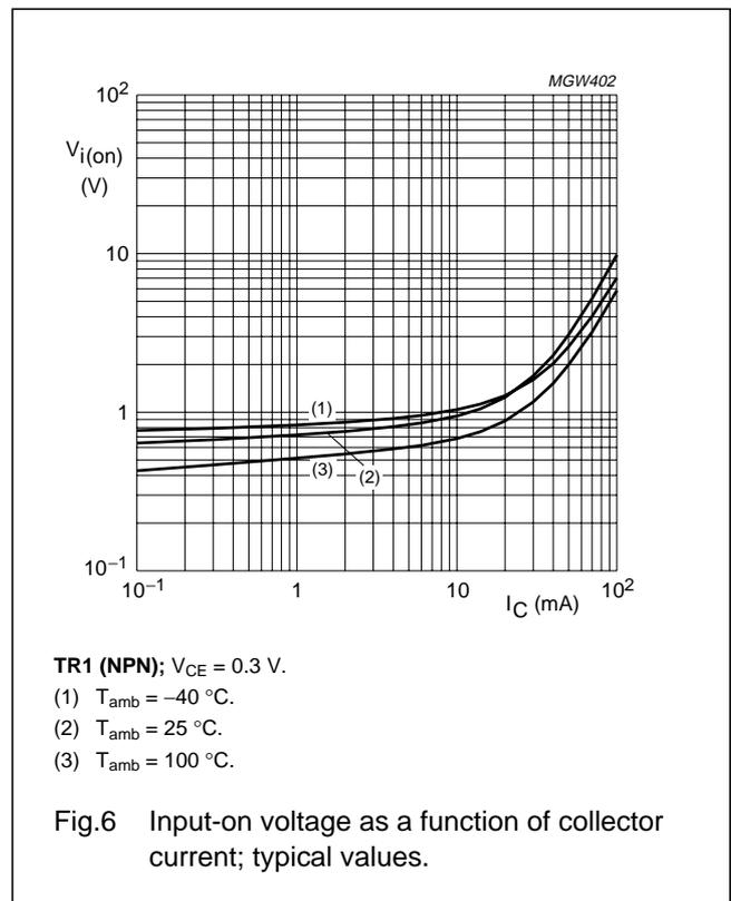
NPN/PNP resistor-equipped transistors;
