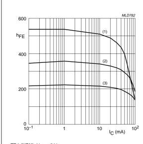
TR1 (NPN);  $V_{CE} = 5 \text{ V}.$
