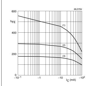
TR2 (PNP);  $V_{CE} = -5 \text{ V}.$
