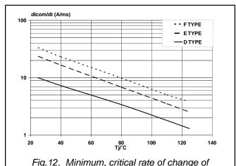
Fig. 12. Minimum, critical rate of change of commutating current  $dl_{com}/dt$  versus junction temperature,  $dV_{com}/dt = 20V/\mu s$ .
