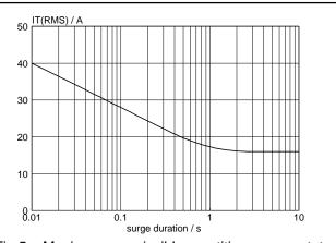
Fig.5. Maximum permissible repetitive rms on-state current  $I_{T(RMS)}$ , versus surge duration, for sinusoidal currents, f = 50 Hz;  $T_{hs} \le 38$  °C.
