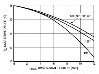
Figure 5. Typical RMS Current Derating
