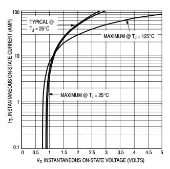
Figure 7. Typical On-State Characteristics
