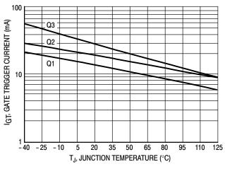
Figure 1. Typical Gate Trigger Current versus Junction Temperature
