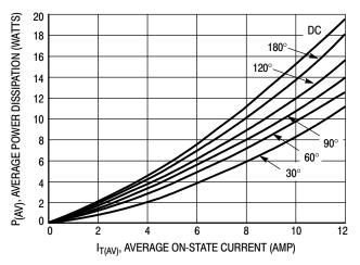
Figure 6. On-State Power Dissipation
