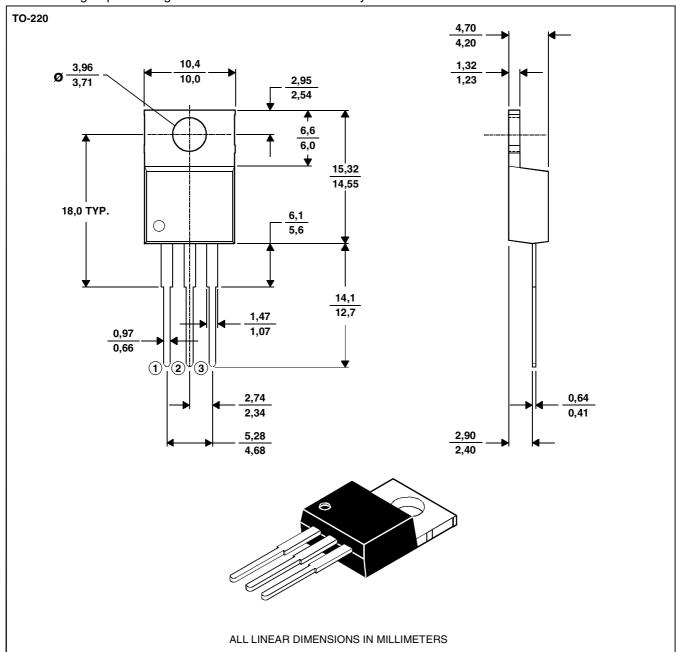
NOTE A: The centre pin is in electrical contact with the mounting tab.
