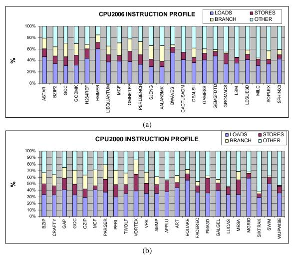
Figure 2-2 (a) Instruction Profile of SPEC CPU2006 Benchmarks (b) Instruction Profile of SPEC CPU2000 Benchmarks
