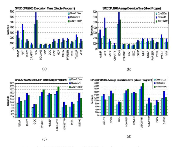
Figure 4-1 SPEC CPU2000 and CPU2006 benchmarks execution time
