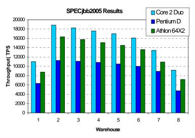
Figure 4-4 Throughput of SPECjbb2005 running with 1 to 8 warehouses.
