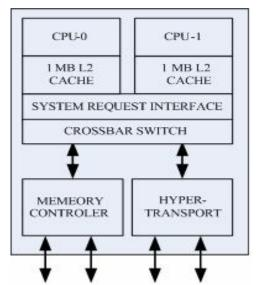
Figure 3-2 Block Diagram of AMD Athlon 64x2 Processor
