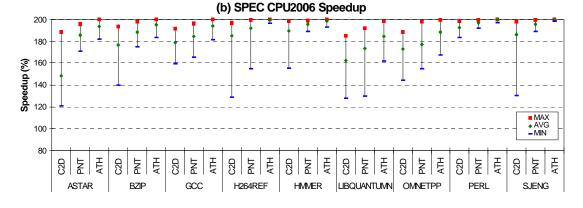
Figure 4-2 Multi-programmed speedup of mixed SPEC CPU 2000/2006 benchmarks.
