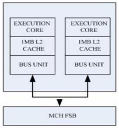
Figure 3-1 Block Diagram of Pentium D Processor
