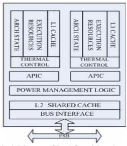
Figure 1-1 Block Diagram of Intel Core 2 Duo Processor
