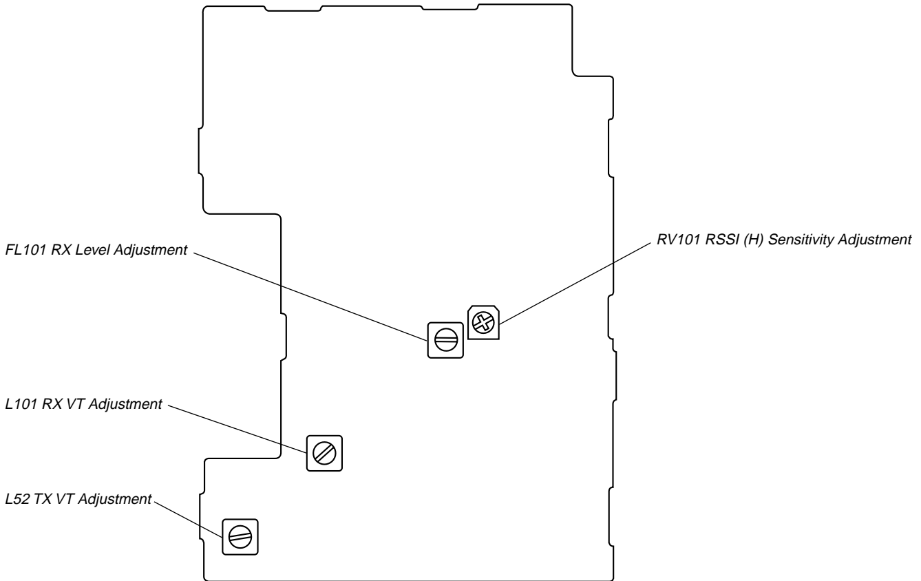
[BASE MAIN Board] (Component Side)
